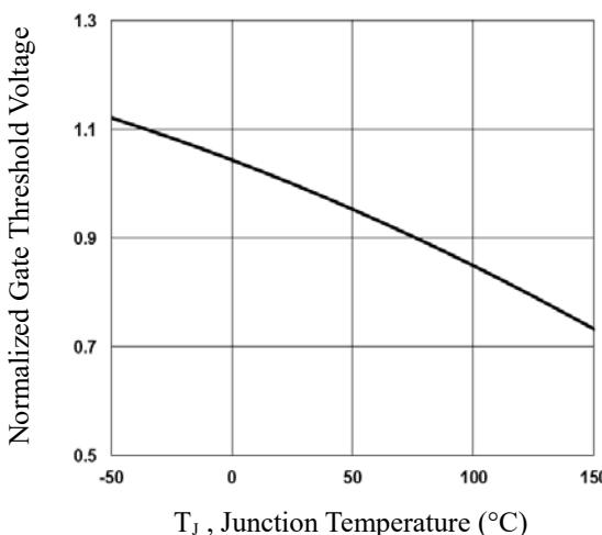
Fig.3 Normalized  $V_{GS}$  vs.  $T_J$
