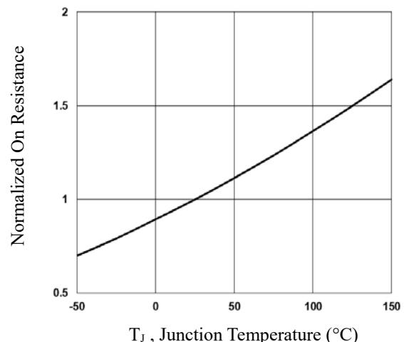
Fig.2 Normalized R<sub>DSON</sub> vs.  $T_J$
